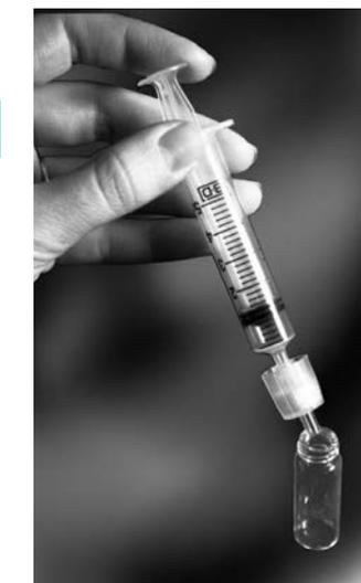
Poly-Pak Cartridge Used Manually
